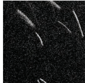
A snapshot of particulates made visible with a dust lamp
